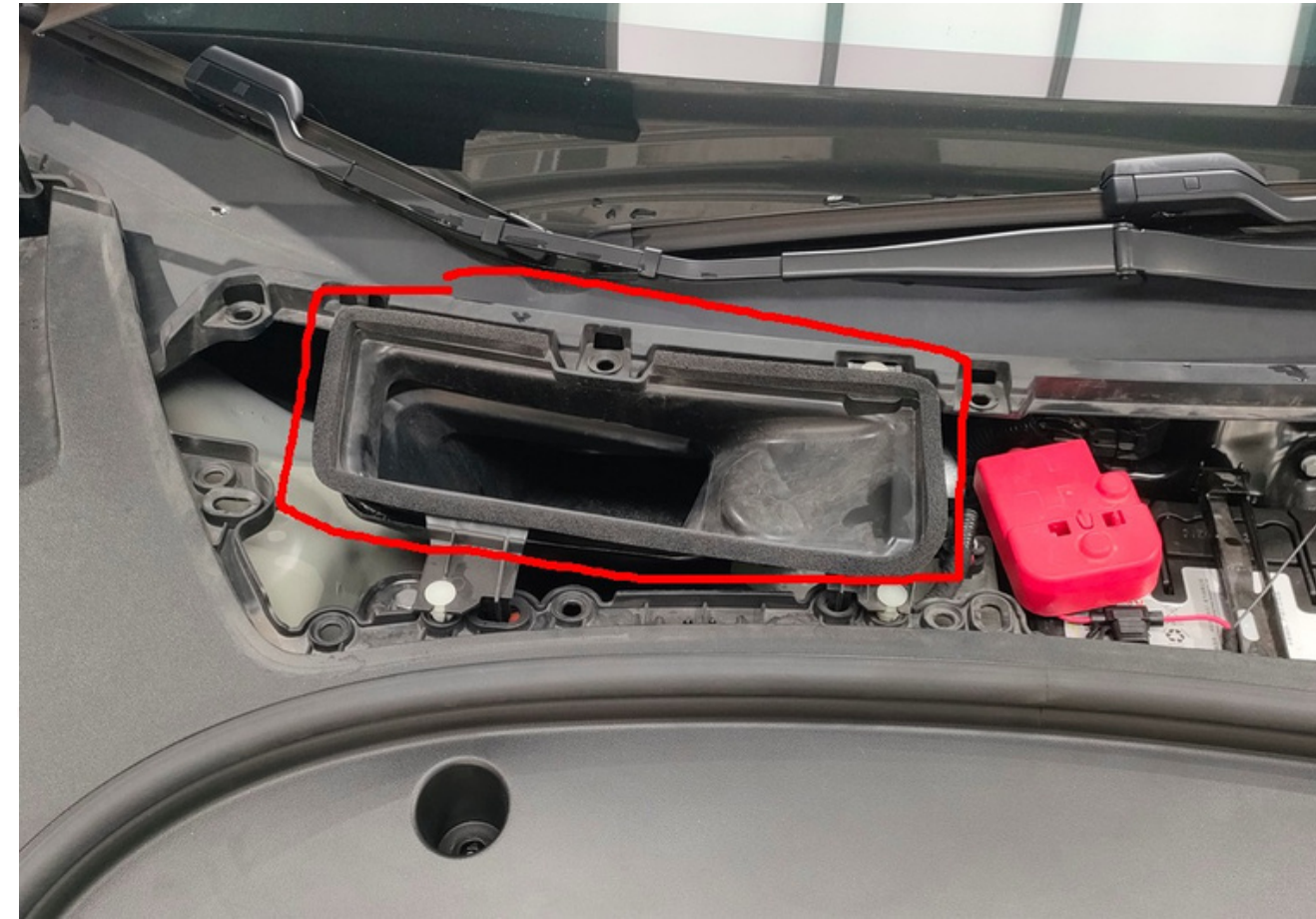
2 Remove ventilation duct (Clips)
